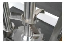
The open axial blade is a specially designed paddle blade that pushes the tank contents downward - Increasing product circulation to minimize mixing time.
