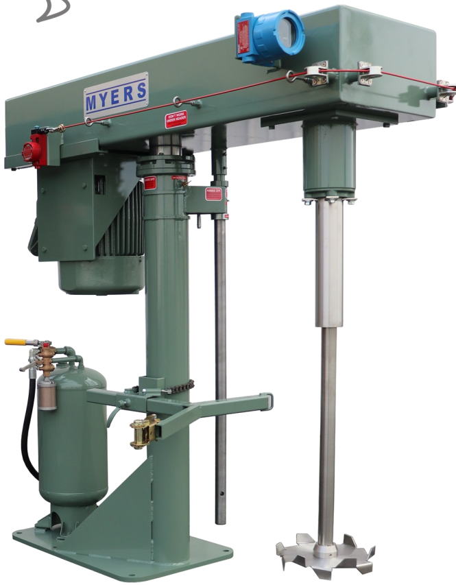
ABOVE: 25 HP explosion-proof model 775 with pipe-style shaft guard, digital tachometer and ammeter, and cable pull limit switch.
