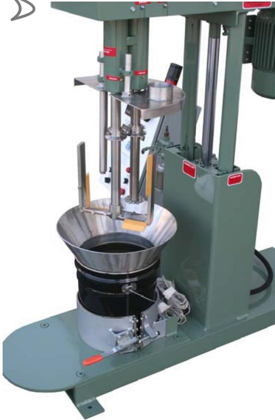
Myers Mixers has designed and manufactured an epoxy resin mixer to handle hot melt epoxies with material process viscosity of 15,000+ cP.
