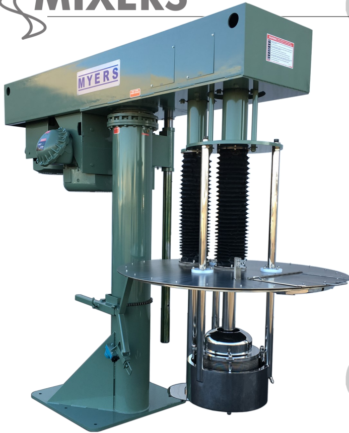
ABOVE: Basket capacity from 1 to 60 liters; the mixer pictured is a 60/30 HP with 38 L basket capacity.
