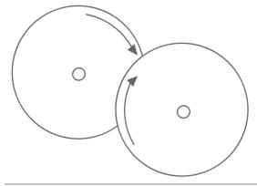
**LEFT:** The overlapping blades are rotating in the same direction. Where the blades overlap, they are moving in opposite directions, effectively doubling the tip speed in this region of extremely high shear.
