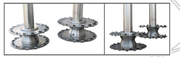
**ABOVE:** The shaft spacing is adjustable. Having the shafts spread provides the most batch circulation. This is important in pigment loading. Having the shafts closed or overlapping provides the best possible dispersion, while reducing batch circulation; this reduces air entrainment.
